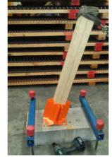
Pic 5 - Safety Base tested to 3160 Newtons without failure
